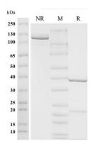
On SDS-PAGE under reducing (R)/non-reducing(N-R) condition. The gel was stained overnight with Coomassie Blue. The purity of the protein is greater than 95%.
